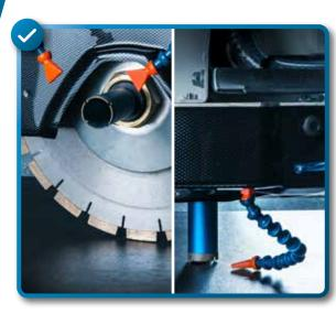
Kw 13 Main Spindle Motor With adjustable speed from 800 till 6000 rpm, complete with interchangeable Easyspin insert with 1/2 gas right thread. It allows the fitting of bit tools with internal water lubrication.
